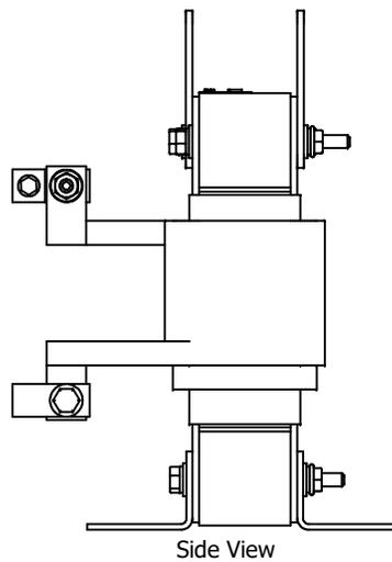
480 Rated Voltage, 600 Max Voltage, High Z, Impedance.
